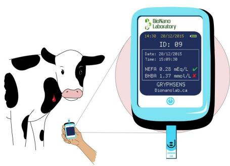
on the nanomaterial based electrode is able to detect the critical clinical range of NEFA and BHBA concentrations in real serum or in buffer samples. This invention (US Serial No. 62/239,474) meets the feasibility of cost-efficient dual sensing at the single electrode chip, with the same blood serum sample.
